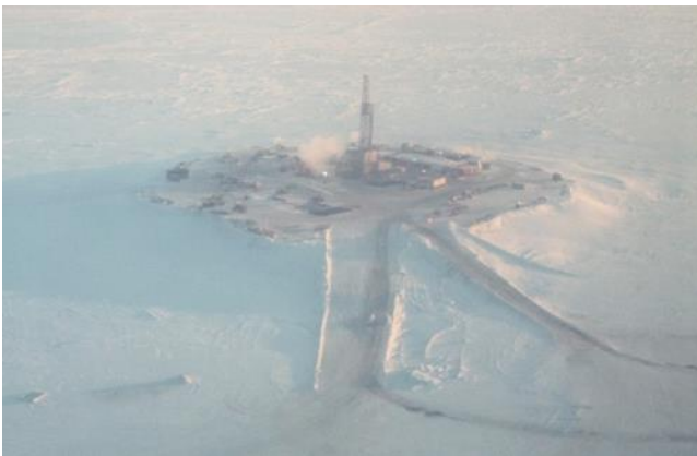
Photo 4: The first exploration well drilled from a spray ice island was from the Mars spray ice island (Early 1986)
