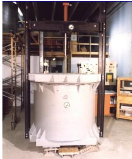
Photo 7: Golder's CPT calibration chamber
