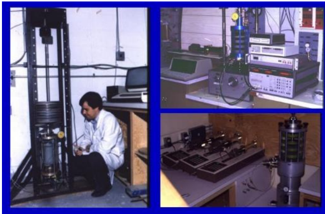
Photo 1: Some of our laboratory testing equipment (Left - early load controlled liquefaction cell; Upper Right – modified triaxial cell to measure dielectric changes during test; Lower Right – GDS computer controlled cell for any stress path or cyclic testing)
